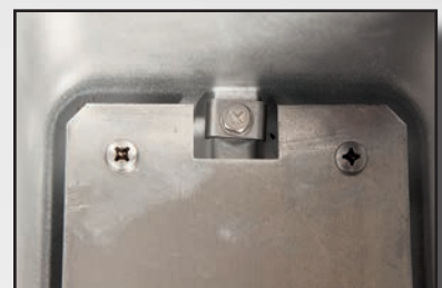
Internal earth screw in body
